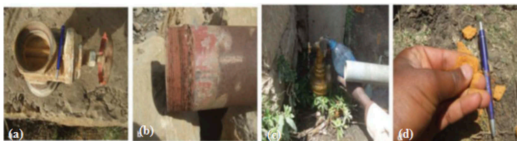
Figure 2. Effect of metallic corrosion: (a) gate valve out of order; (b) thread of pipe damaged; (c) gate valve starting to scale and rusting; and (d) metallic material, pipe, almost changed into soil due to corrosion (Source: Corrosionpedia.com).
