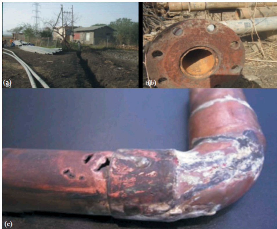
Figure 1. Effect of corrosion on metallic material: (a) replacement of metallic pipes by PVC after leakage and clogging problems; (b) corrosion problem on metallic pipe joints; (c) pinhole leaks in copper tubing caused by internal corrosion (adapted from McFarland et al. 2011).
