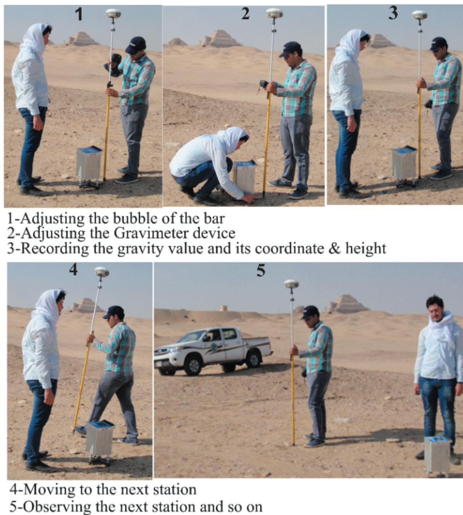
Figure 5. The research team accurately measures the gravity and position of the grid points.
