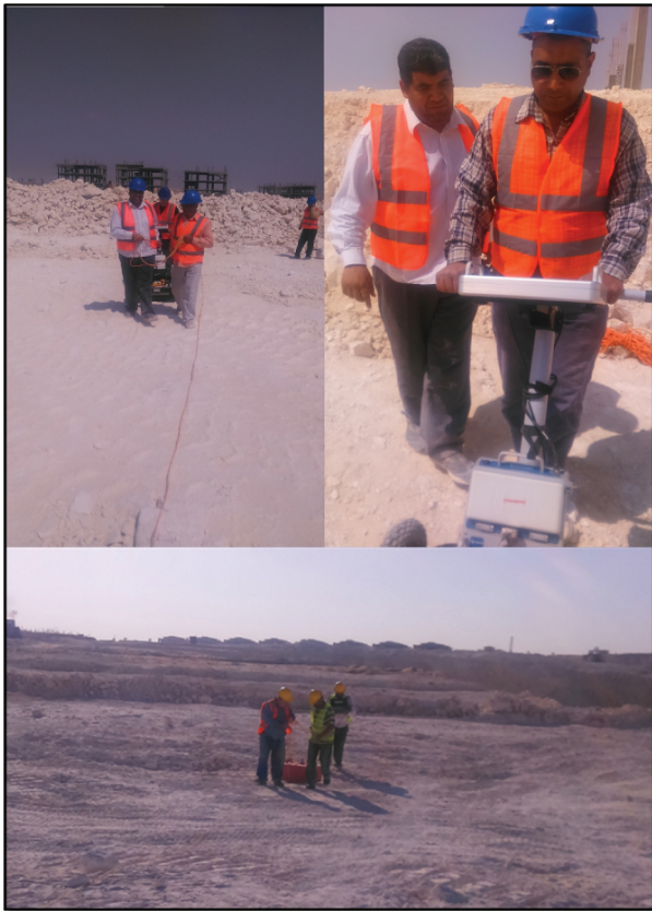
Figure 5. The GPR scan with SIR 4000 and Mala systems using 200 and 250 MHz antennas during acquisition.
