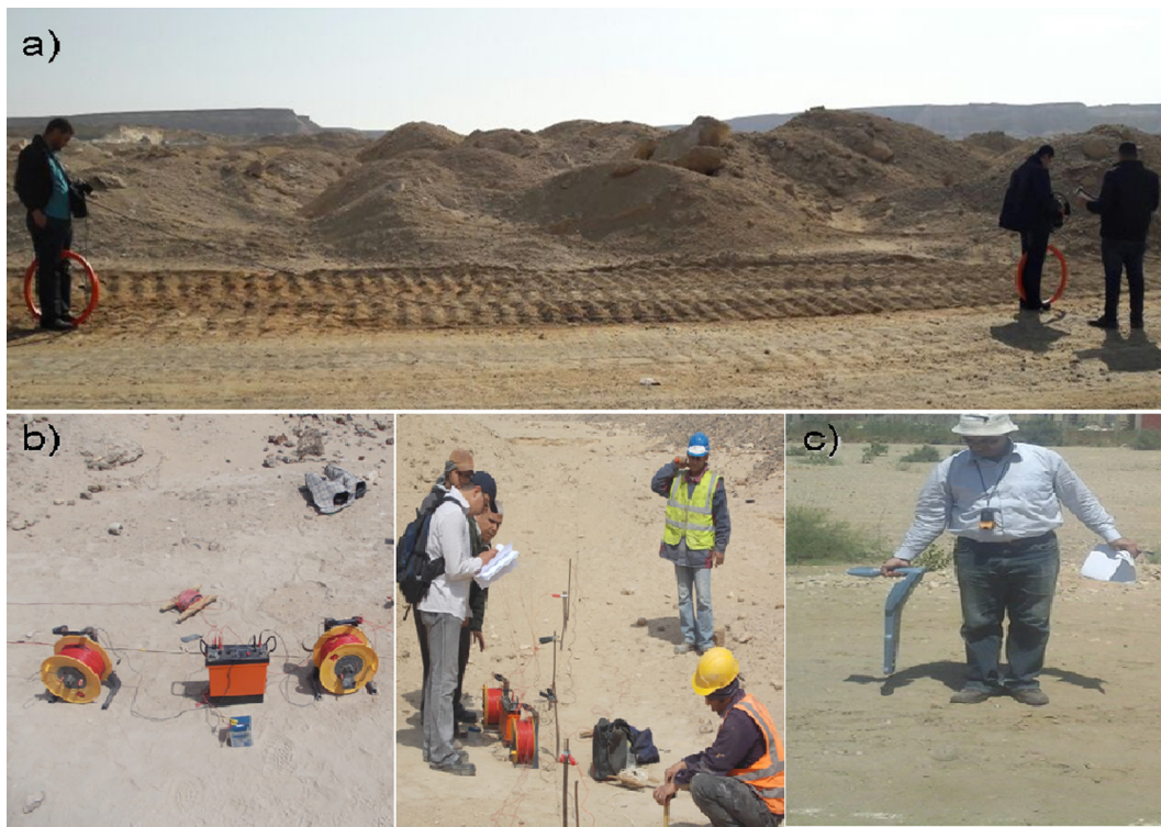
Fig. 4. Field photographs showing the (a) Geonics 'EM-34-3', (b) ABEM 'Terrameter-SAS-300C' and (c) RadioDetection 'RD-8000' measuring systems.
