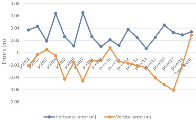
Fig. 7. The differences between the point clouds derived by RTK-DG and the point clouds derived from AT process.
