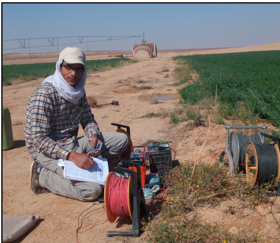
Fig. 4. Data acquisition using Terrameter SAS 1000 resistivity meter instrument.
